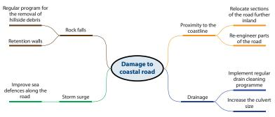
Figure 2-4: Cause and Effect Diagram
