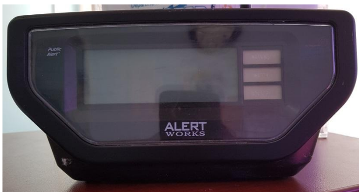
Picture 3: Showing a NOAA weather radio receiver. These units offer slightly less functionality than RDS receivers (they cannot display alert text) but they do provide alert audio and are very affordable.
