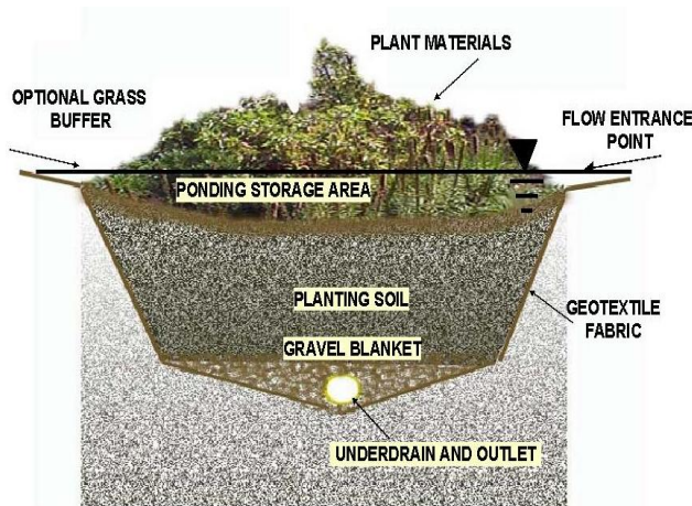
Figure 2: Cross Section of Retention Cell/Rain Garden
