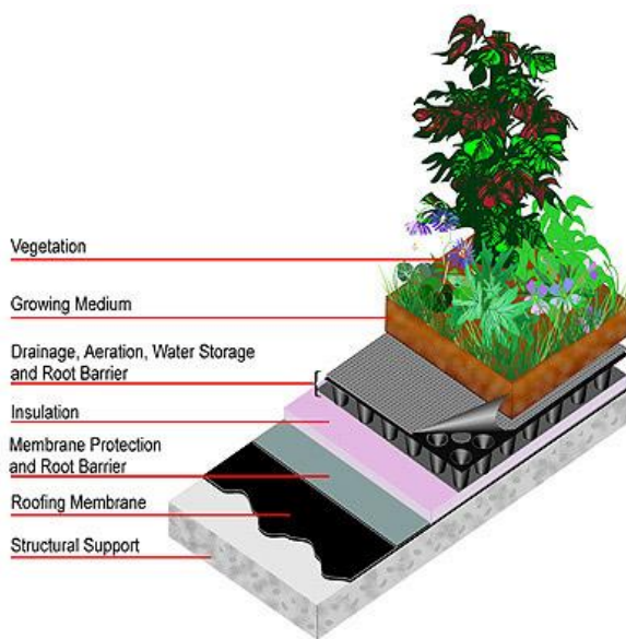
Figure7: Typical Green Roof
