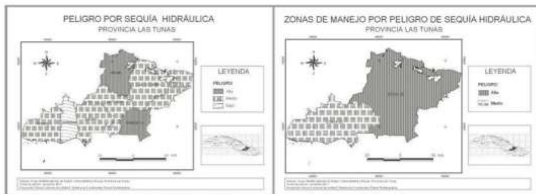
Figure 4.6: Hazard map; a) Hydraulic Drought, b) Management of hydrological drought hazard, for Las Tunas province.
